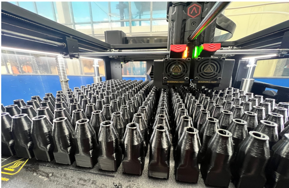
Bed of Wiring harness parts being Printed on the Raise3D Pro 3 Plus
